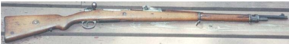
Belgium, Mauser Belgian Mod. 1889 Rifle, 1889, Bolt Action, 5 shot Integral Mag, Charger strips, 7.65 mm Mauser, 8.9 lb.
