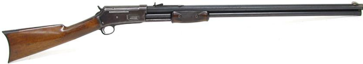
USA, Colt Lightning Slide Action Rifle, 1887-1894, Pump action 15 shot tub mag under barrel, .45-65 cal, 9 lb.
