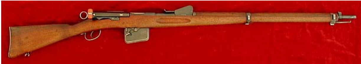
Switzerland, Schmit-Rubin Mod 1889 Rifle, 1889, Bolt Action, 12 shot Removable Clip, 7.5X53 mm, 10.7 lb, 51.2" overall
